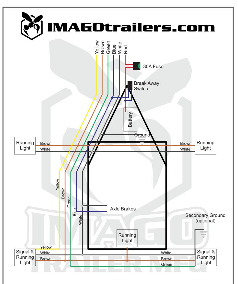
The wiring schematic provided is for our dump trailer models DT7000, DT10000, DT12000, DT14000 and DT21000. This schematic should be used for American destined trailers only. Please contact IMAGO Trailer Manufacturing if you are an international customer, as your wiring may be different due to your tow vehicle's specifications.
